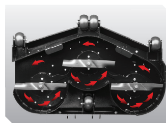
48", 54", and 60" Decks – Deep 7 gauge shell to tackle deep grass
